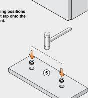
5. Insert drawer front adjusters manually or with a MINIPRESS insertion ram (MZM.0095)
