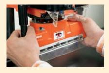
An optional 7 or 8 spindle boring head can be used for boring 32 mm system hole groups and can be used for drawer front boring and assembly.
