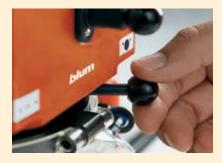
5 spindle swiveling head Multiple patterns are achieved by turning the head 90°.
