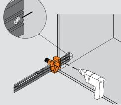
Aligning for mounting plates/adapter plates
