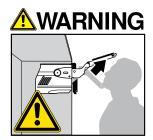
Lever arm can spring up and cause injury without door attached
